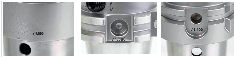
Fig. 6: Marking for checking of the clamping force: Three possible positions on the hydraulic chuck
