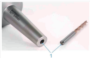
Fig. 8: Cleaning hydraulic chuck and tool
