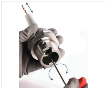
Fig. 10: Adjusting the tool length
